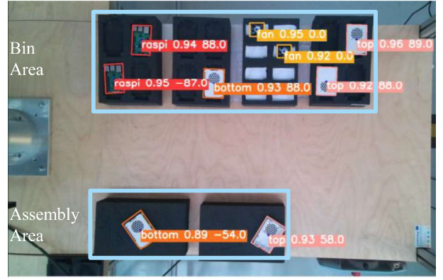
Fig. 8. Top view on the workstation and object detection result.
