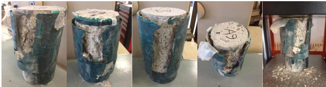
Fig. 1: Break shape of confined concrete.
